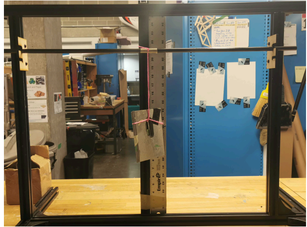
Figure 7.6.2: (left) Theoretical and (right) Measured Deflections for Three-Point Load Test and Three-Point Load Test Setup
